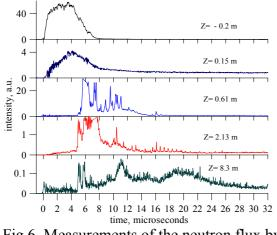
Fig.6. Measurements of the neutron flux by "local" detector. At Z= -0.2 m detector registered bremstrahlung of the beam only.  $n_0=1.9\cdot10^{21}$  m<sup>-3</sup>.
