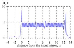
Fig.1. Configuration of the magnetic field.
