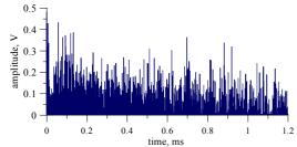
Fig.4. Waveform of signal of digital PSD stilbene detector of fusion neutrons (Z=4.3 m). Initial deuterium density is  $1.9 \cdot 10^{21}$  m<sup>-3</sup>.
